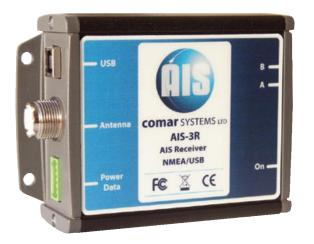
The AIS-3R is a high performance, dual channel AIS receiver, with outputs for both NMEA 0183 and USB. The AIS-3R reads and decodes all AIS messages that are specified and transmitted by AIS Class A and Class B tranponders, AIS SARTs and Aids to Navigation. The AIS targets together with all the static and dynamic information received can be displayed on any AIS compatible Chart Plotter or PC navigation program.
